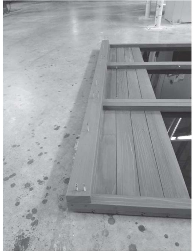
Apply the trim to the outside where the three panels meet. Peel off the paper masking of the double sided tape and place the trim over the center of the joint. Press firmly to apply.
